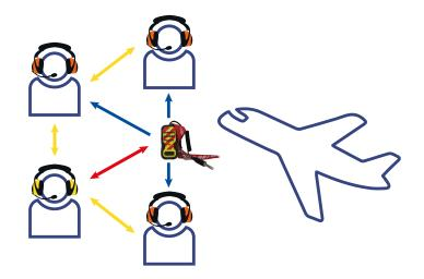
Moreover, the 3 positions of the PTT allows you to choose which position allows communication with the cockpit: the UP position only allows communication with operators, the MIDDLE position turns off the microphone and the BOTTOM position allows communication with anyone (operators + cockpit).
